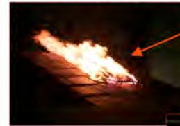
Burning [12"x 12"] 'A Brand' placed on roof covering. Will flame penetrate through the covering to the underside of the roof deck (into the attic), or not?
