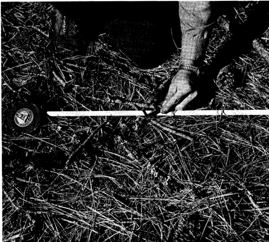
Figure 3.--Diameter of the intersected twig is checked with a go-no-go gage. The plot rod marks the sampling plane.
