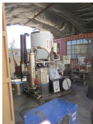
HEF members investigate alternatives such as an on-site power pallet gasifier/generator from a local Berkeley company.
